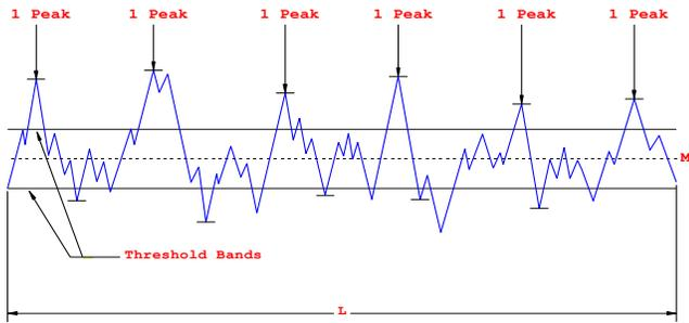
**Peak Density,  $P_c$** , is the number of SAE peaks per unit length measured at a specified peak count level.
