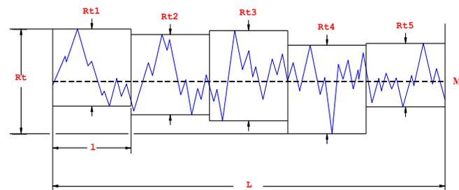
**Maximum Height of the Profile,  $Rt$** , the vertical distance between the highest and lowest points of the profile within the evaluation length.
