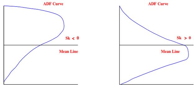
**Skewness,  $R_{sk}$** , is a measure of the asymmetry of the profile about the mean line. A negative skewness indicates that a greater percentage of the profile is above the mean line and a positive value indicates that a greater percentage is below the mean line.
