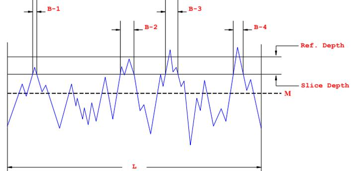
**Profile Bearing Length Ratio,  $t_p$** , the ratio of the profile bearing length to the evaluation length at a specified level.
