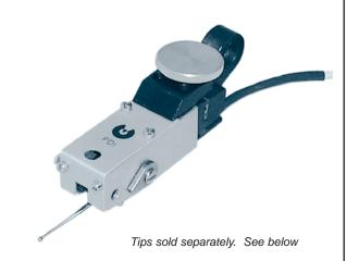
**T-425 Gage Head**, lever type, breakaway feature to protect tips. Includes adjustment wrench. Has fine mechanical adjustment of 0.045" (1.14mm) for standard gage tips and 0.090" for 2X. Gaging force: 0 to 0.5g over a gaging range of  $\pm 0.020$ " for standard gage tip; with 2X tip: 0 to 0.3g force over a range of  $\pm 0.040$ ".
